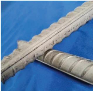
图 1 双相体不锈钢钢筋 Fig. 1 Duplex stainless steel reinforcement
