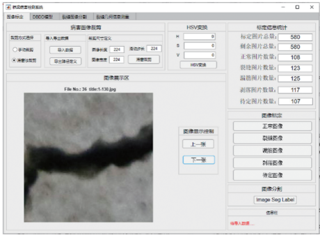
图 7 基于 Matlab GUI 设计简易的病害图像裁剪及标定工具箱 Fig. 7 Design a simple disease image cropping and calibration toolbox based on Matlab GUI
